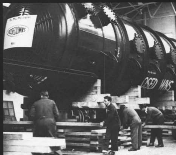
The largest Deodoriser in Europe with a capacity of 20,000 lbs/hr. being prepared for dispatch.
